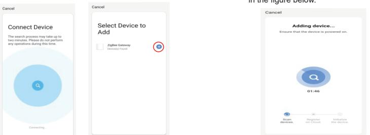
7. After adding the Zigbee gateway, click the gateway to enter the device addition page
