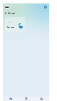
8. Switch to "Zigbee device list" as indicated in the figure below, then click to add a device.
