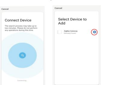
6. The mobile phone enters the device search and connection mode as shown in the figure below.
